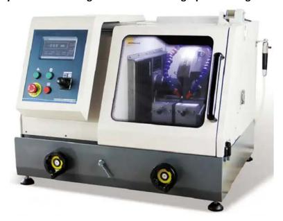
Model AC-100/AC80 cutting machine is composed of main machine, electric control box, cutting room, motor, cooling system, cutting grinding wheel and other parts.
